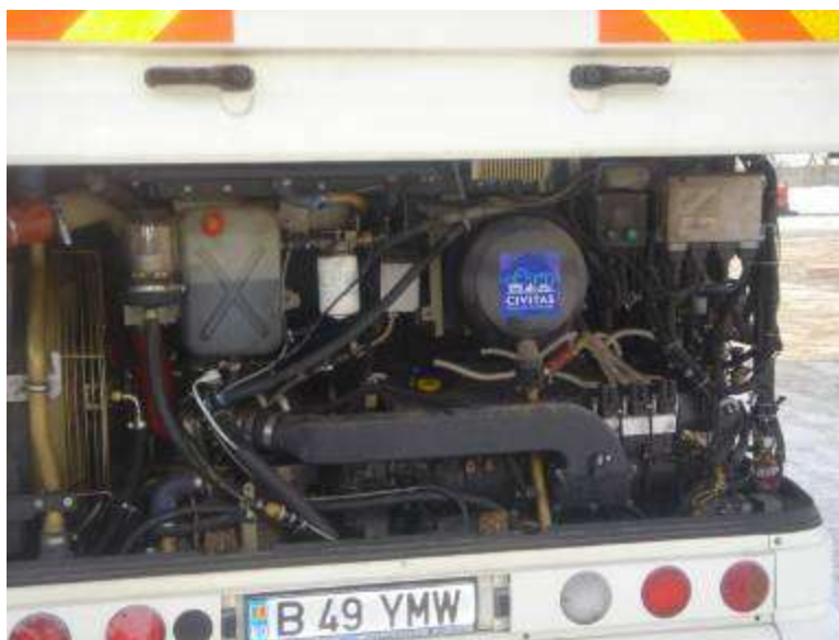
Figure 11: LPG converting system on a bus
