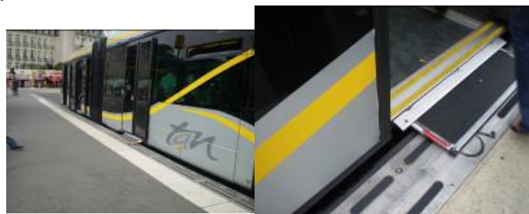
Ramp for mobility impaired access
