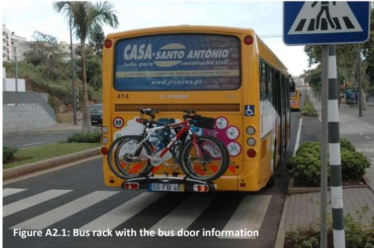
Figure A2.1: Bus rack with the bus door information
