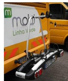
**Figure B2.1: Bus rack installed on a Green Line bus**
