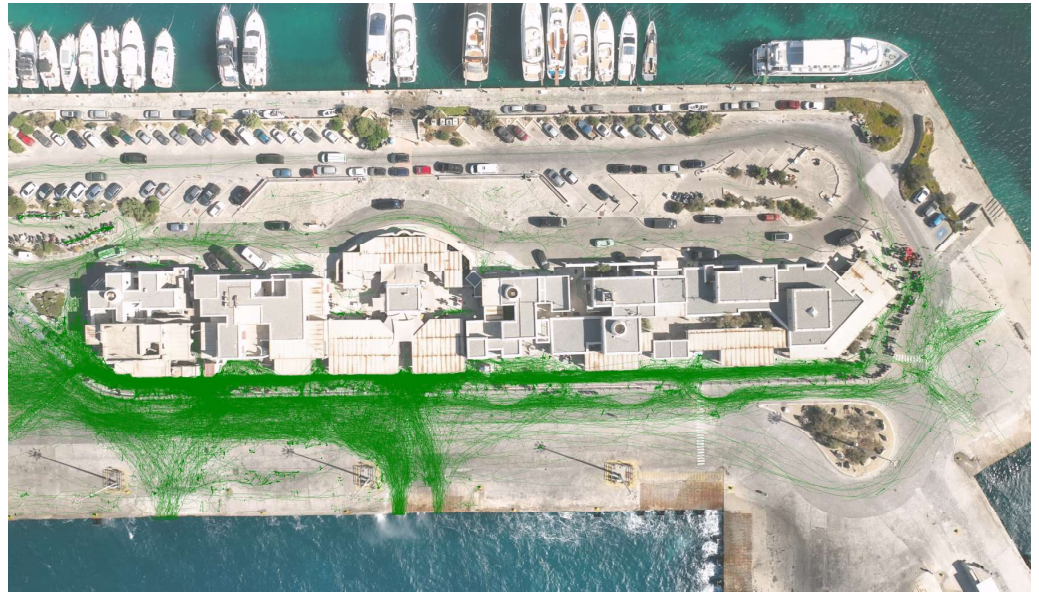
Figure 6. Pedestrian trajectories (represented in green lines) at the Mykonos port dock recorded between arrival and departure of two boats.
