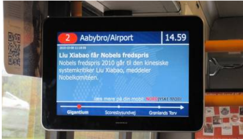
Figure 1: News display (the upcoming bus stops and the destination are always displayed)
