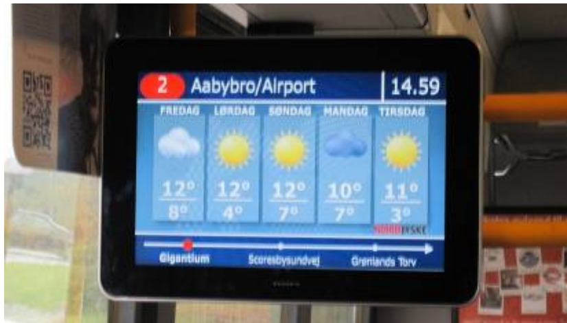
Figure 2: Weather forecast display (the upcoming bus stops and the destination are always displayed)
