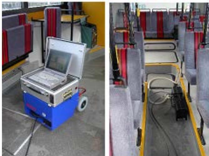
**Figure 3: Mobile testing equipment. Left picture shows 5-gas analyser with battery box and PC. Right picture shows the opacimeter with sample tubes directed through the cabin floor to the exhaust.**
