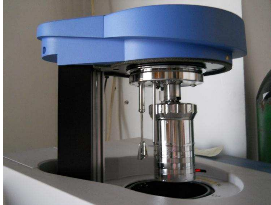
Figure 6 – Equipment for the energy content measurement
