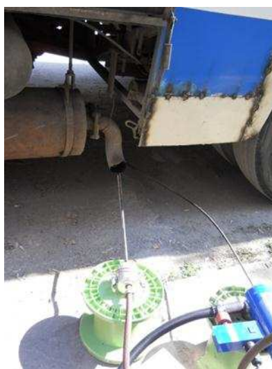
Figure 4 – Measurement of emissions at tailpipe
