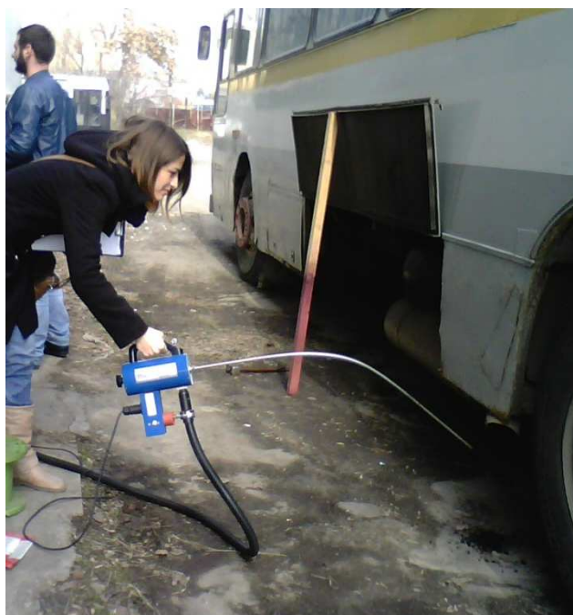
Figure 8 – Measurements of emissions at tailpipe
