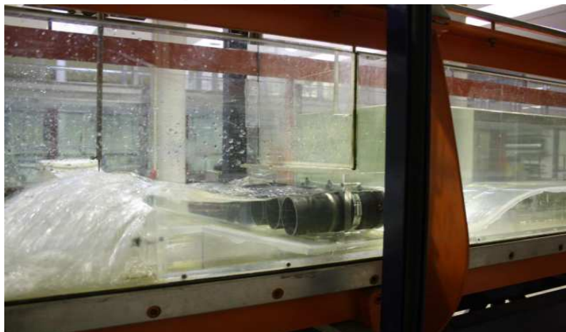
Fig. 5 - Laboratorial tests considering 3 turbines in a scale model of the Coimbra Dam spillway sill.
