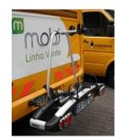
Figure B2.1: Bus rack installed on a Green Line bus
