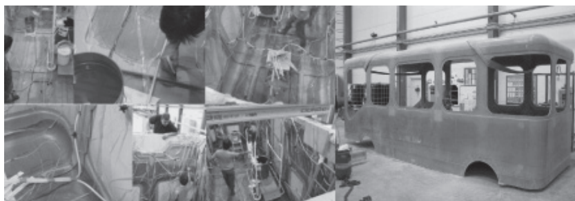
Figure 11: Bodywork part manufactured (infusion by SCRIMP).
