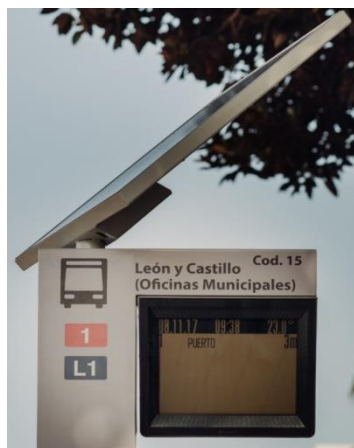
Figure 36: LPA 7.3 - Real Time Information Display and Solar Panel
