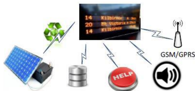
Figure 26: MAD 7.3 - Components of the New Information Panel with Photovoltaic Power
