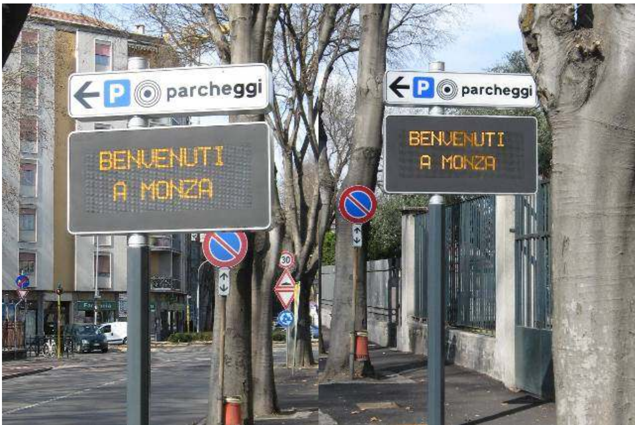
Figure 8 - Infoparking signs with VMS panels
