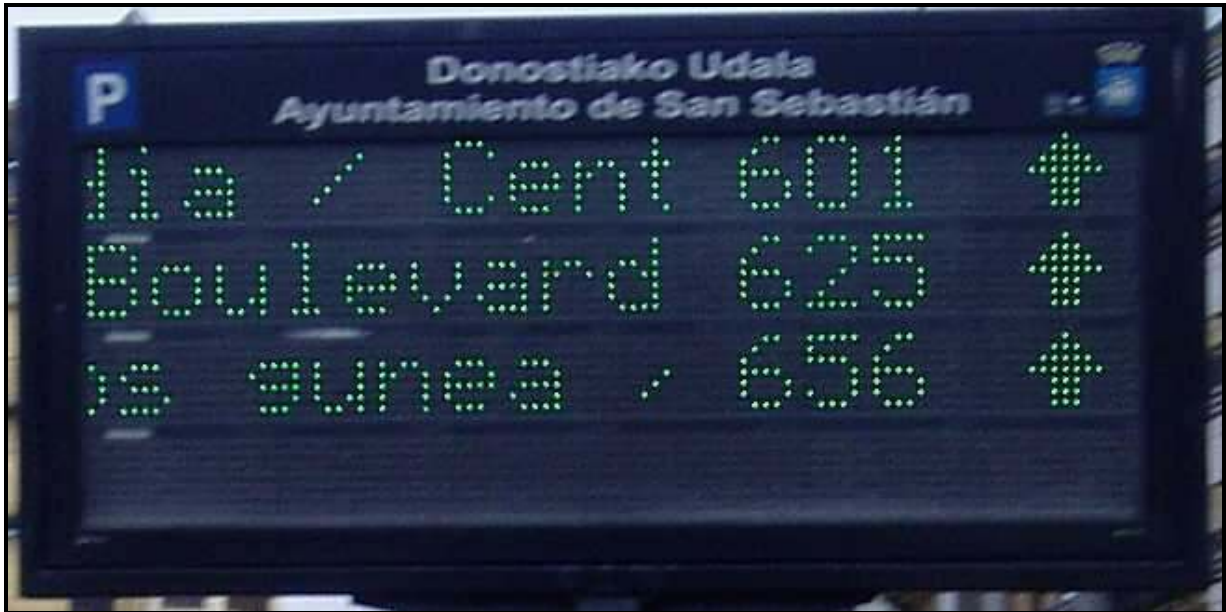
Fig 10. Example of the display lines in a VMS panel
