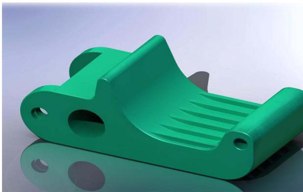
**Figure 2. Individual 'paddle' element of the ramp**
