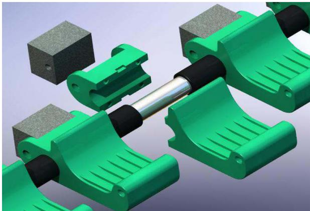
**Figure 3. Image showing how the ramp elements connect to each other**
