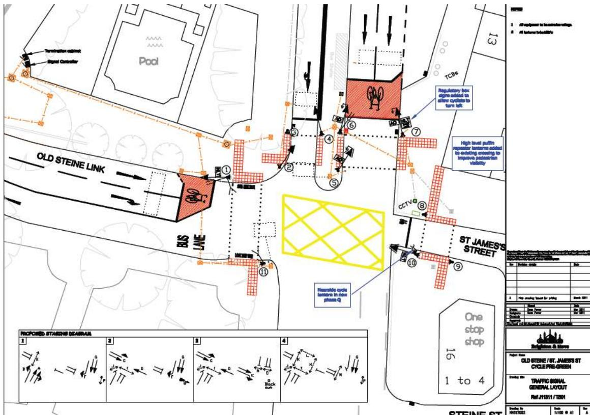
Figure 5. Design drawing for the cycle left turn signals
