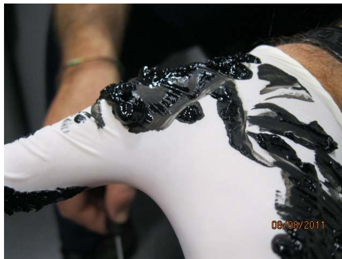
Figure 1: Waste taken from the fuel filter walls
