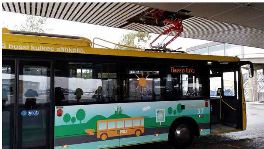
Figure 1: Electric bus charging
