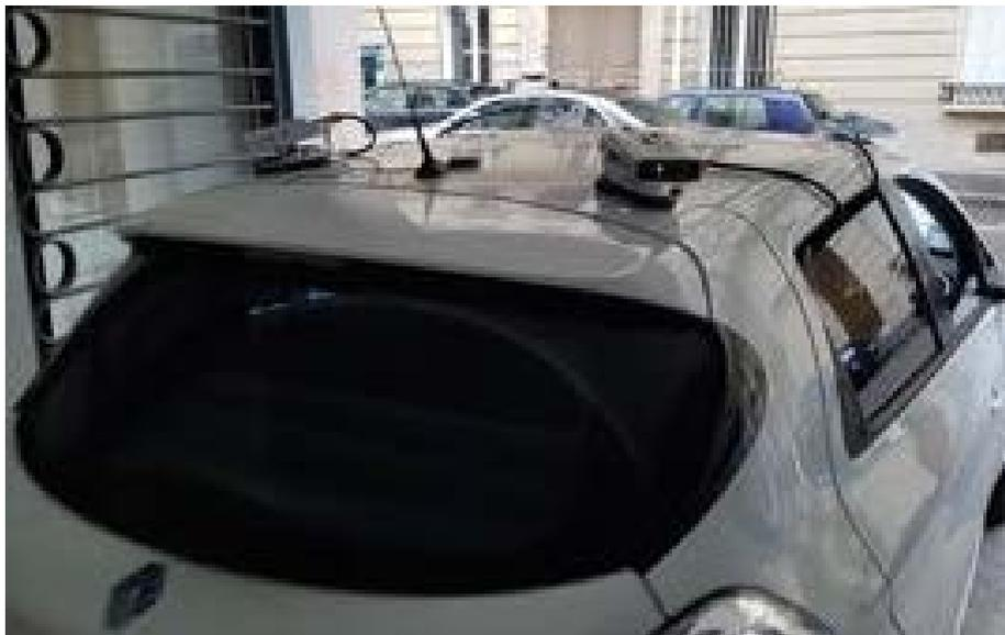
**Figure 3:** STO 2.4 technical equipment parking scan car (left) (Source: City of Stockholm)
