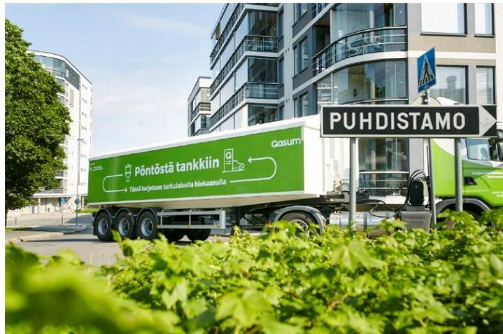
**Figure 6: Heavy duty vehicle fuelled by liquefied biogas (LBG) from wastewater sludge**
