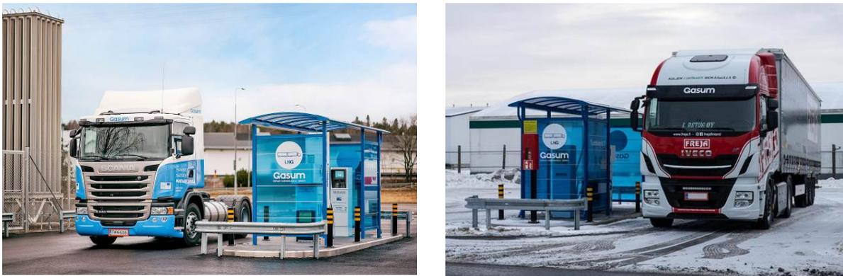
**Figure 7: LBG trucks and associated fuelling station**
