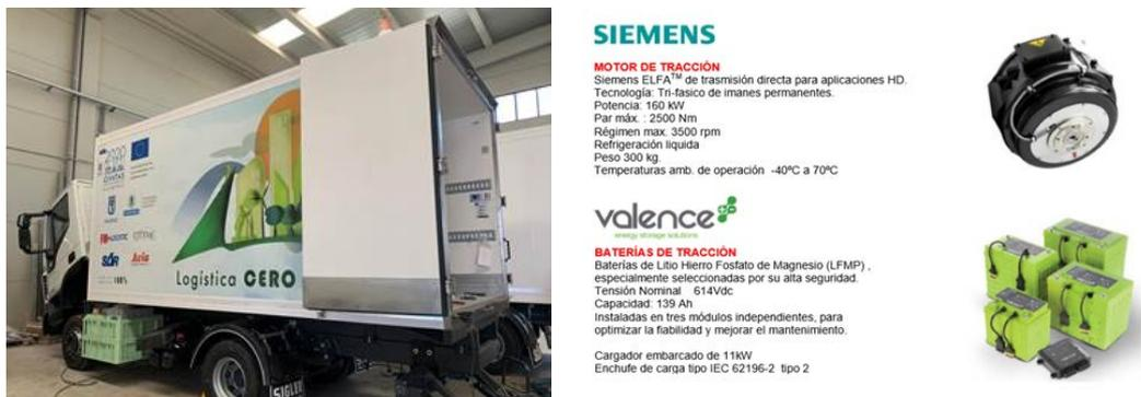
**Figure 3: Bodybuilding and main components of the electric truck prototype**
