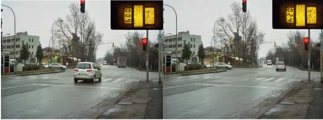
Figure 1 and Figure 2 – STARS: the system takes two photos of each vehicle passing while traffic light is red
