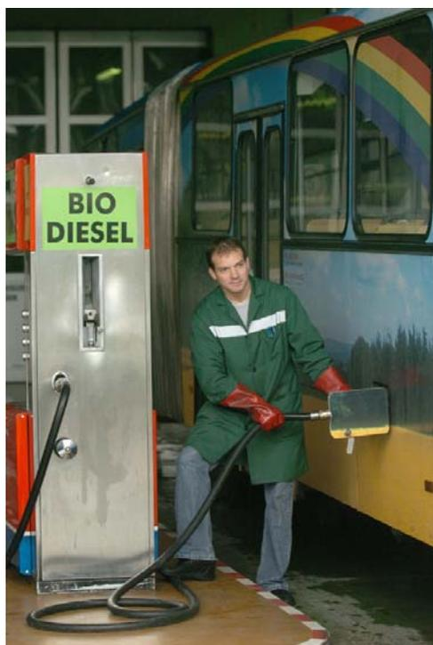
After using a mixture for a period of two months the laboratory test results concluded that water was extracted from the fuel mixture and therefore the quality of fuel is not suitable for further use. Because of that and warnings from the fuel supplier, Petrol, that some chemical reactions can take place in fuel mixture which can cause damage to engines, LPP decided to use 100% biodiesel.
