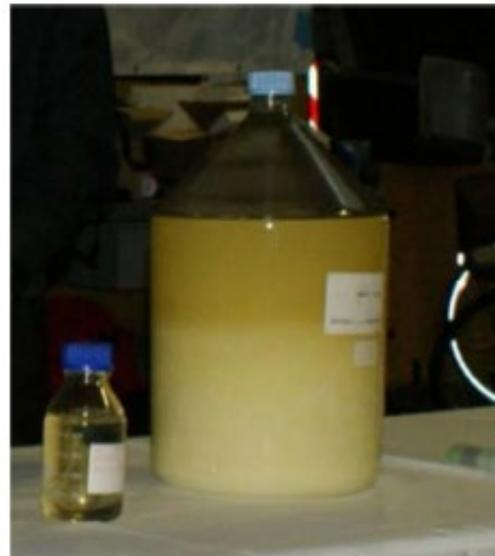
**The affect of colder temperatures on 100 % TME. To the left is TME in temperatures of 5-10 °C and to the right is TME in temperatures of -5 - 0 °C. Note the difference in transparency.**
