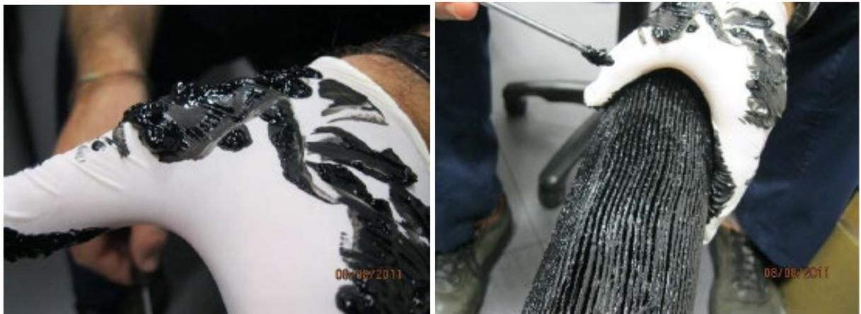
**Initial problem with saturation of fuel filters affecting buses with common fuel injection system in Donostia-San Sebastián.**
