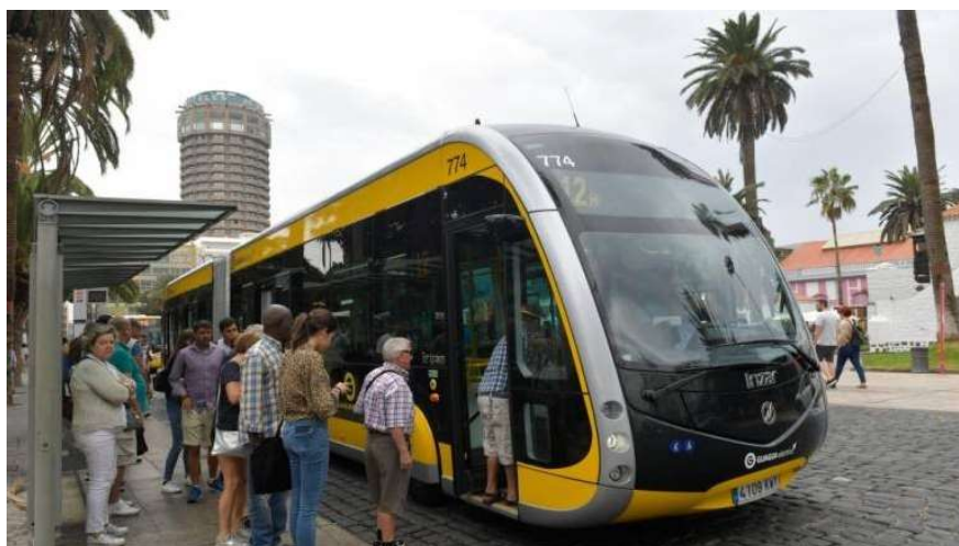
Figure 13: Fully electric articulated bus (Irizar ie-Tram)
