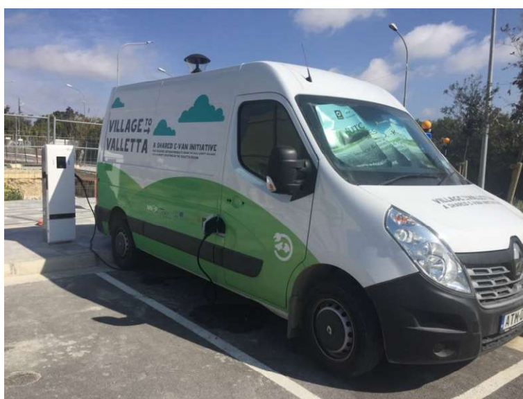
Figure 7: The electric van used for goods delivery in the pilot project
