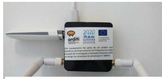
Figure 3: Smart OpenWrt based sensor / router used to track mobility trends (with 4G mobile data pen)
