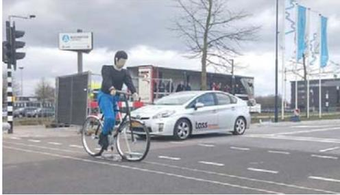
The intersection is provided with a radar which the presence of cyclists detect. This information is transmitted via a dedicated Wi-Fi network. The approaching car picks up the signal, before the cyclists are visible to the driver and then the brakes works automatically.
