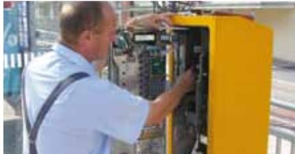
The first ten vending machines were equipped with wireless modems as part of the testing phase. These modems automatically send a message to the control centre if there is a problem.
