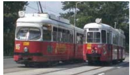
Upon first evaluation, energy consumption was found to have declined by 35 percent. Known as a chopper system, the upgraded trams are assisted by an on-board computer and application that processes energy consumption. The system transforms kinetic energy into electrical energy, which is recovered in the power line and consumed by other vehicles. A more comfortable and safer journey is also provided thanks to a smoother start-stop phase.
