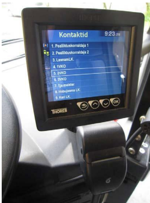
Figure 1 Driver communication unit
