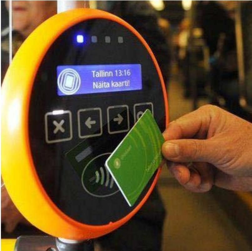
**Figure 1 Contactless card validator**
