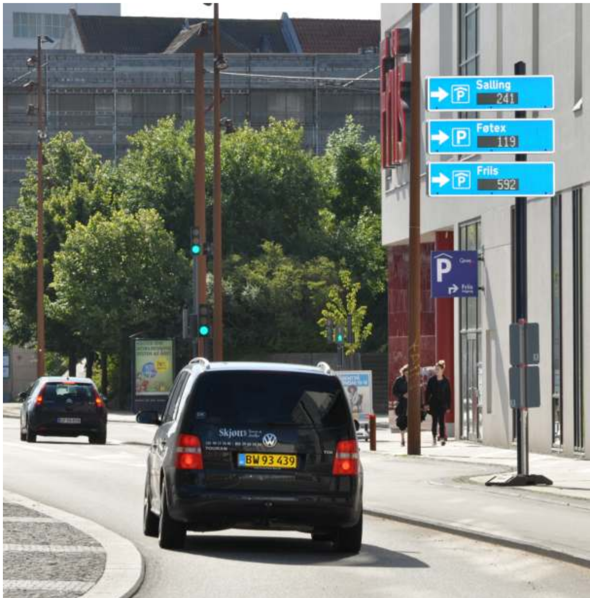
Figure 5 Dynamic sign, showing free parking spaces in three different car parks. All these private.
