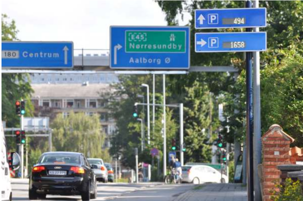
Figure 4 Dynamical sign in the periphery of the city centre showing free parking spaces in two different parking zones of the city centre.
