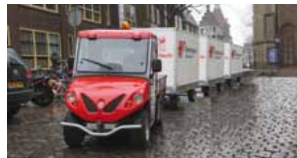
The cargohopper is a 16-metre long electric vehicle that delivers goods around Utrecht
