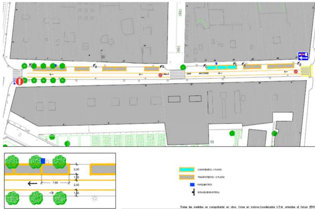
Figure B4.5: Sample area of proximity in San Antonio Street integrated with traffic calming measure and bicycle line.
