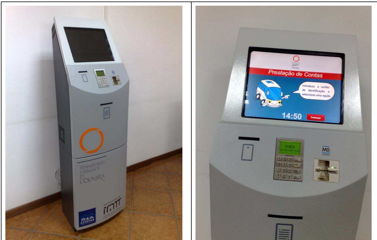
Figure B4.2 - The automatic machines for PT drivers account activities is allowing the payment by ATM of the results of the tickets sales on board buses with economies of resources on the accounting office
