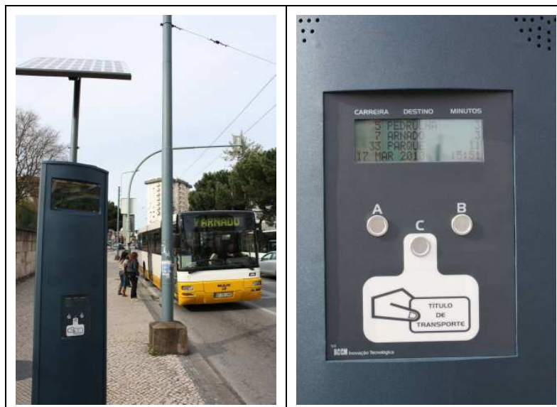
Figure B1.1 – Real time information panel at bus stops powered by solar energy (left) and detail of the secondary module with second information screen and “contact less” reader (right)
