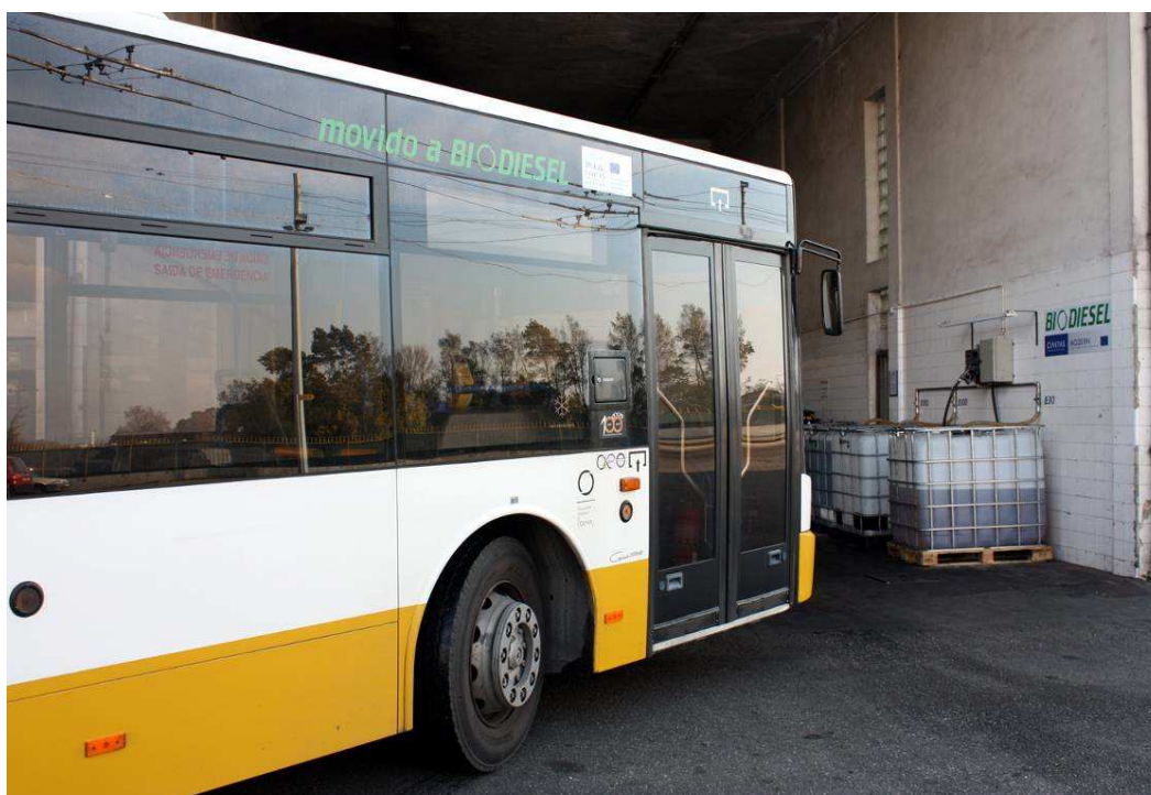
Fig. B4.2 – Bus approaching the bio fuel refuelling area equipped with the reservoirs and pump. The bus has stickers informing that is running with bio fuel.
