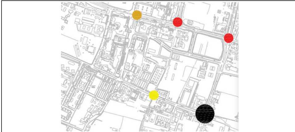
Fig. 5 Extract of the map showing the dangerousness of the road intersection based on the count of the number of accidents occurred in the reference period. The more the colors are dark and the more the intersections are dangerous.
