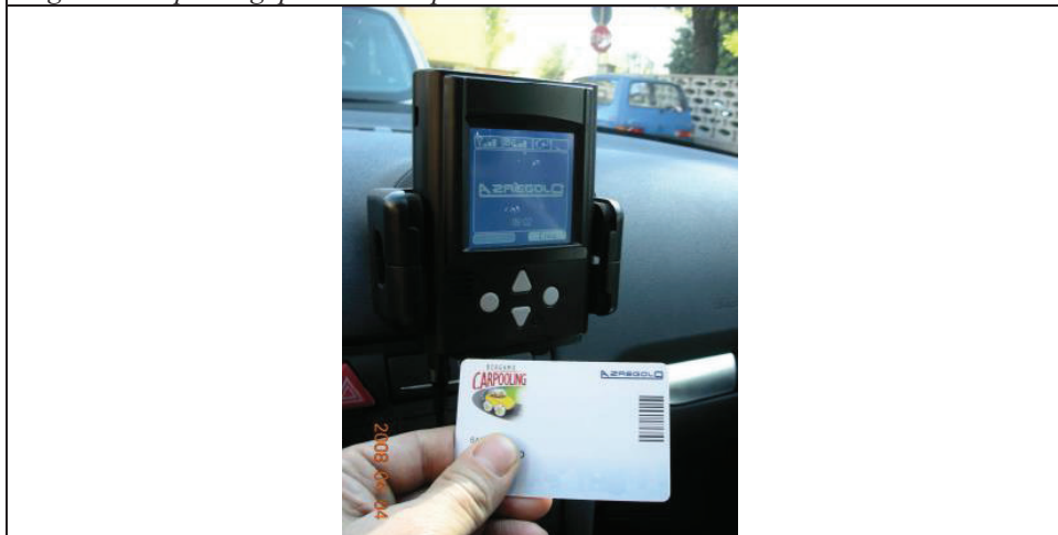
Fig.3B: Data logger device to be installed on board provided by the company AZ Mobility for the CAR-POOLING experimentation in Brescia
