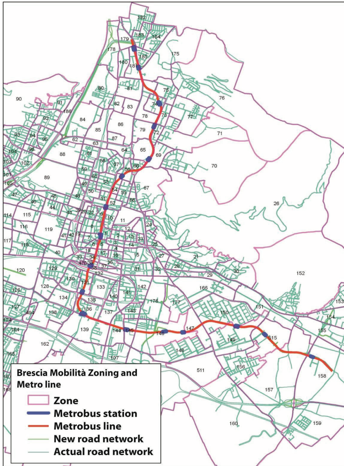
Fig.A4.2: New zoning of the city of Brescia used to build up different scenarios
