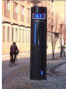
Pictures 2A and 2B: One of the two bicycle “barometers” in Malmö. Sensors are located under bicycle lane. Barometer displays number of cyclists that have passed on that day (1633 so far on this day) and in “bars” indicates monthly and yearly totals to date. There are two displays on opposite sides of the barometer so that cyclists, pedestrians and motorists can see from either direction.
