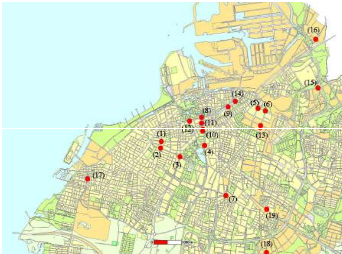
Map 2: Plans for the installation of Bicycle Radar Detectors during Stage 2 (2006). Detector 14 was included in the full study in the spring of 2008. Furthermore, detectors 8, 11, 10 and 4 were passed by cyclists in “test runs” to measure effects of passing several detectors in a row along a bike lane.
