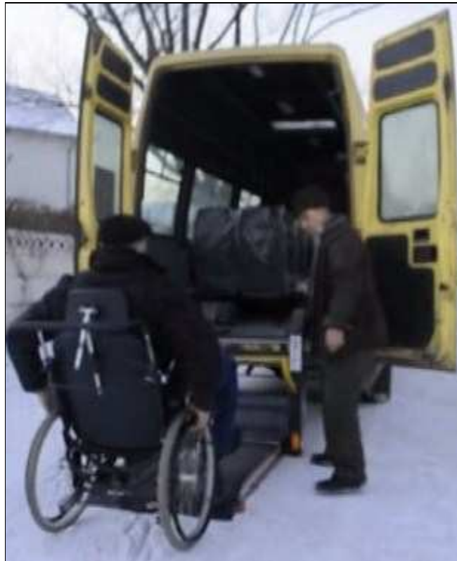
Figure 4: Electro hydraulic lifting platform within different positions
