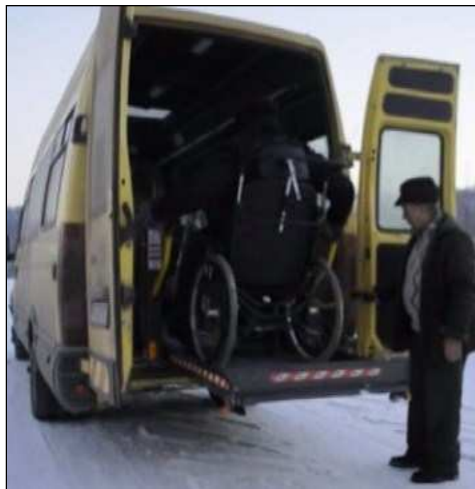
Figure 5: Electro hydraulic lifting platform within different positions
