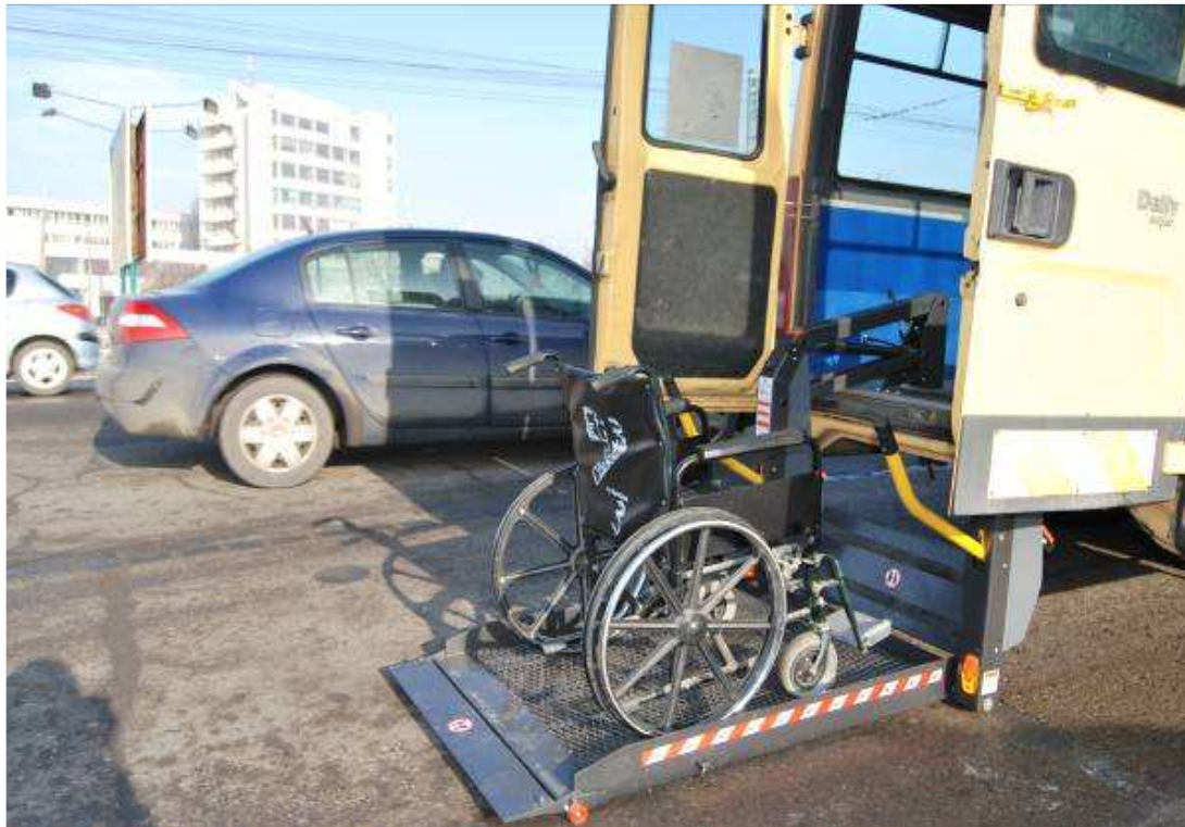
Figure 1: Electro hydraulic lifting platform within different positions
