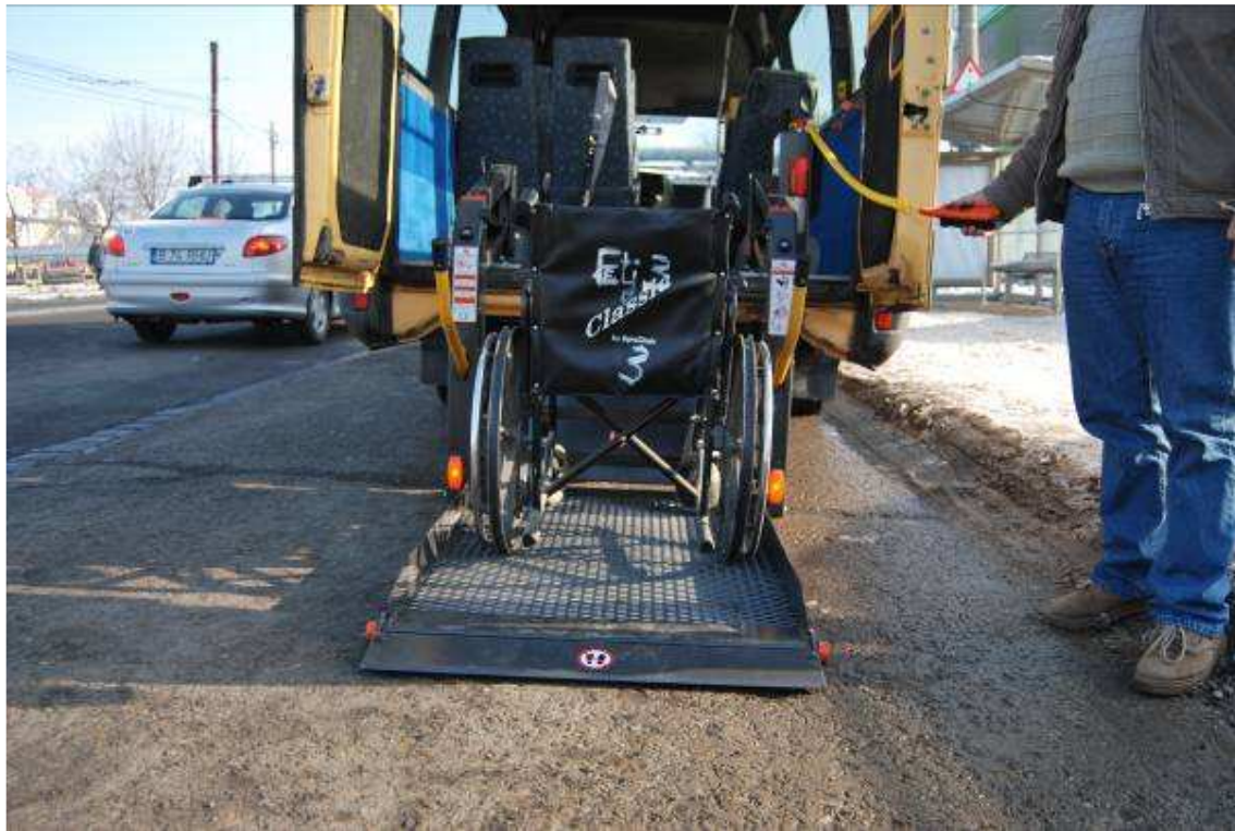
Figure 2: Electro hydraulic lifting platform within different positions
