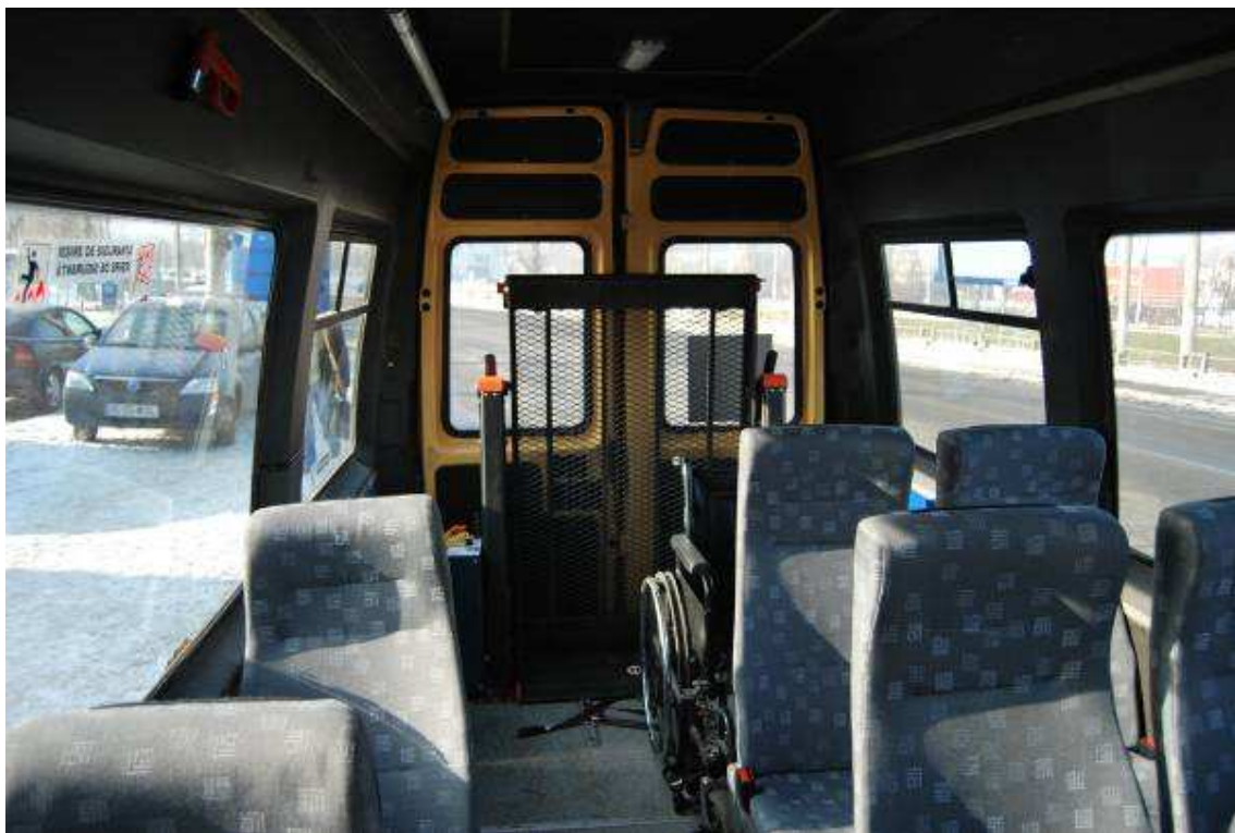
Figure 3: Electro hydraulic lifting platform within different positions
