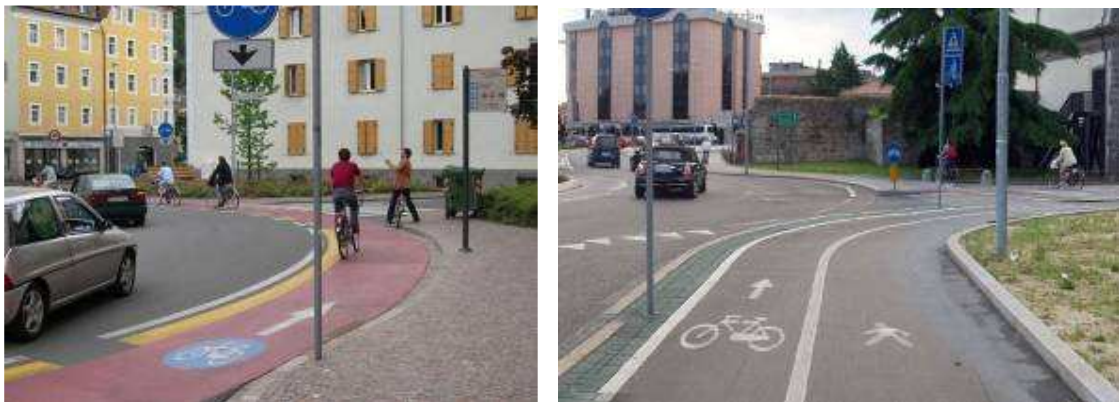
Figure 3 - Examples of cycling routes in roundabouts
