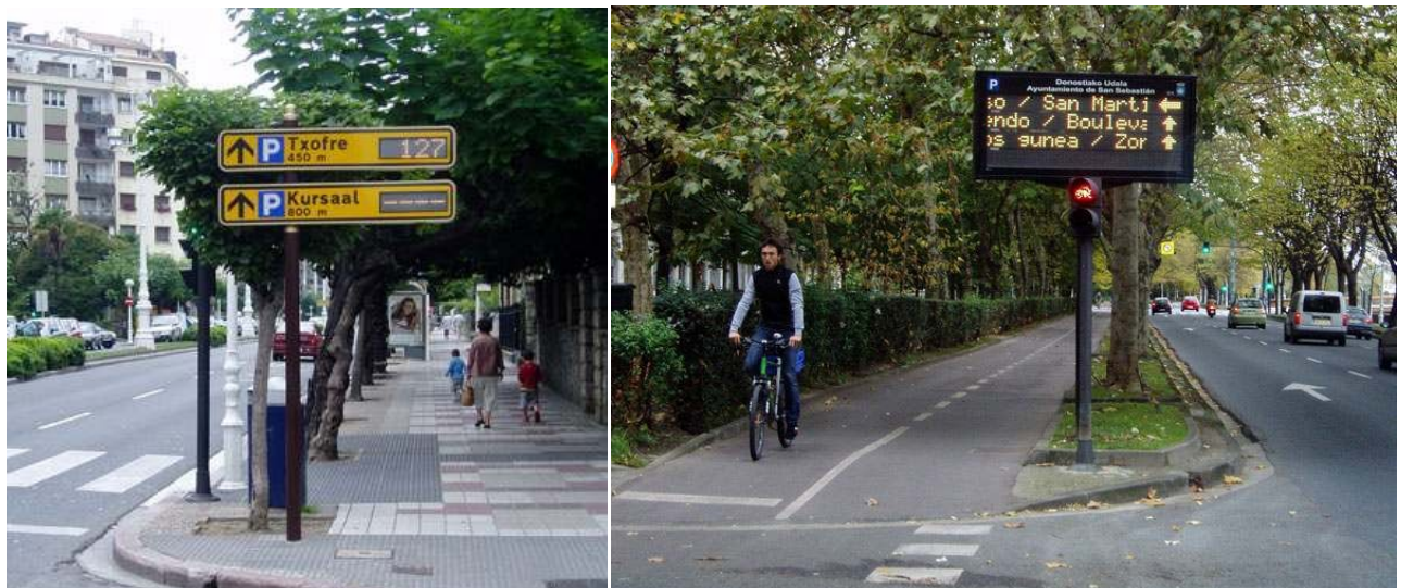
Figure 5: The parking guidance system in Donostia - San Sebastián consists of signposts (pictured left) and variable message signs (pictured right).
