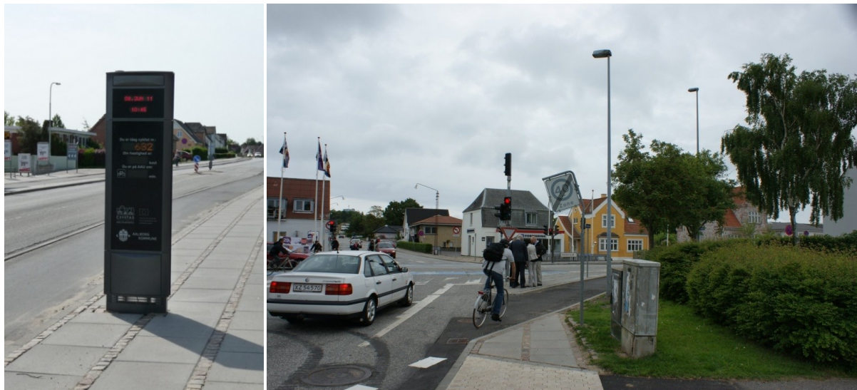
Figure 5: The bicycle counter (pictured left) and the segregated bicycle filter lane (pictured right) are both part of the cycle motorway in Aalborg.
