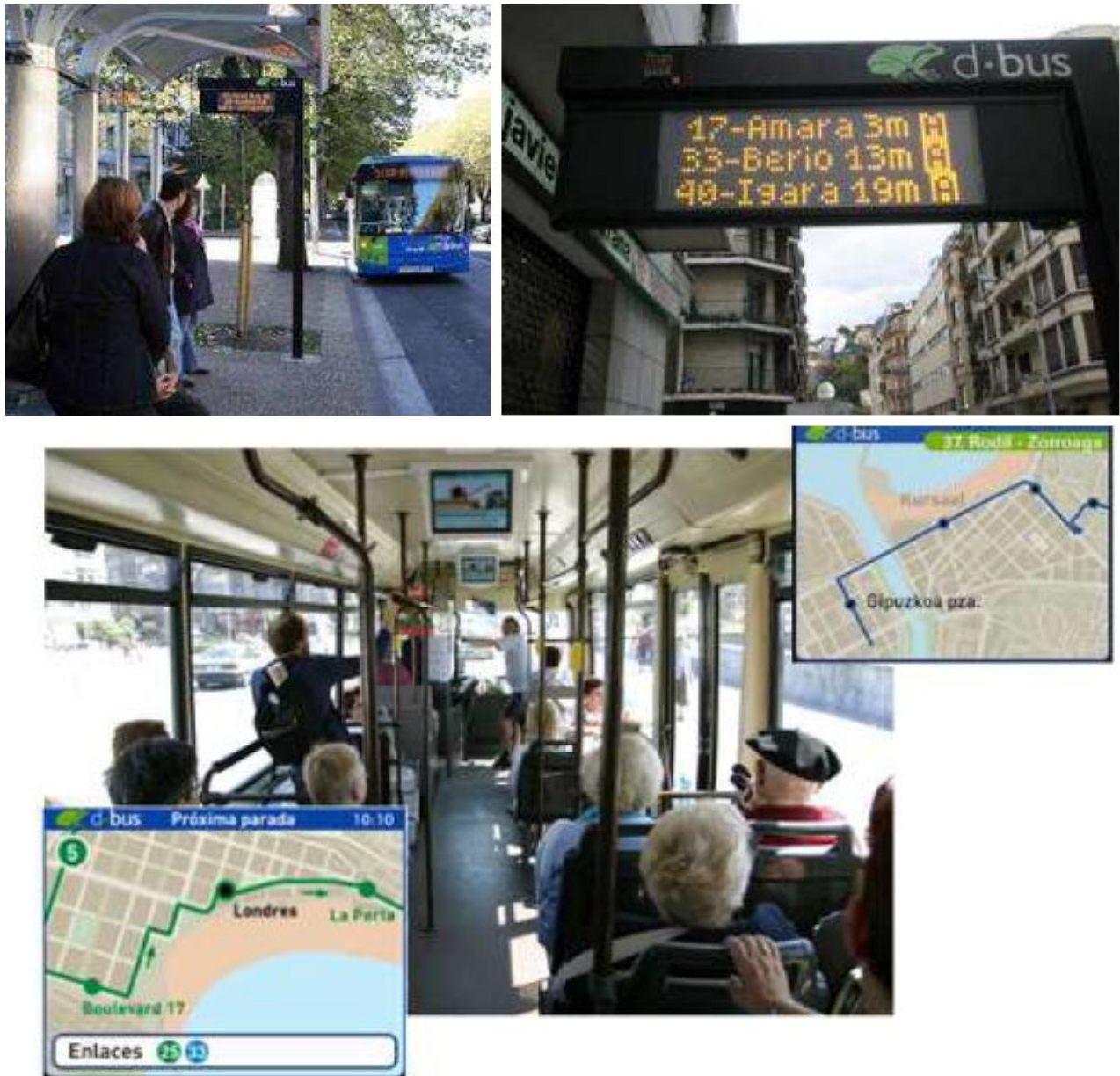
Figure 3: New real time information at bus stops and onboard information system with next stop announcement in Donostia - San Sebastián.
