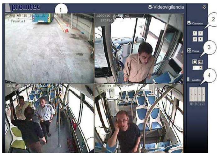
On-line video visualization of the bus in the control centre transferred by HSDPA-3G communications
