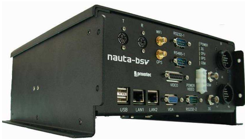
HSDPA-3G modem included in the advanced computer for video administration and managing (onboard the bus)
