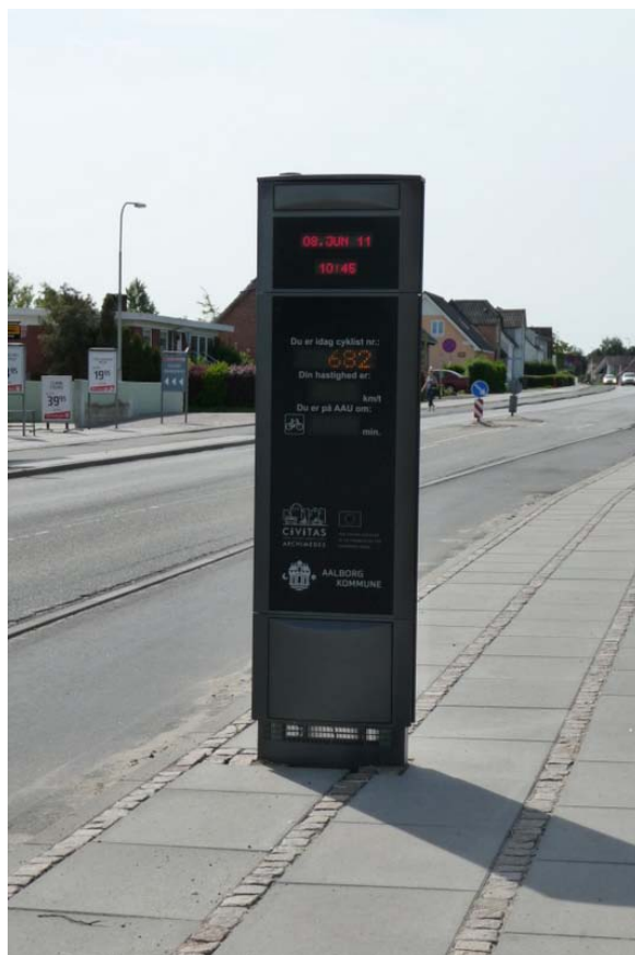
Figure 6: The bicycle counter installed at the cycle motorway.
