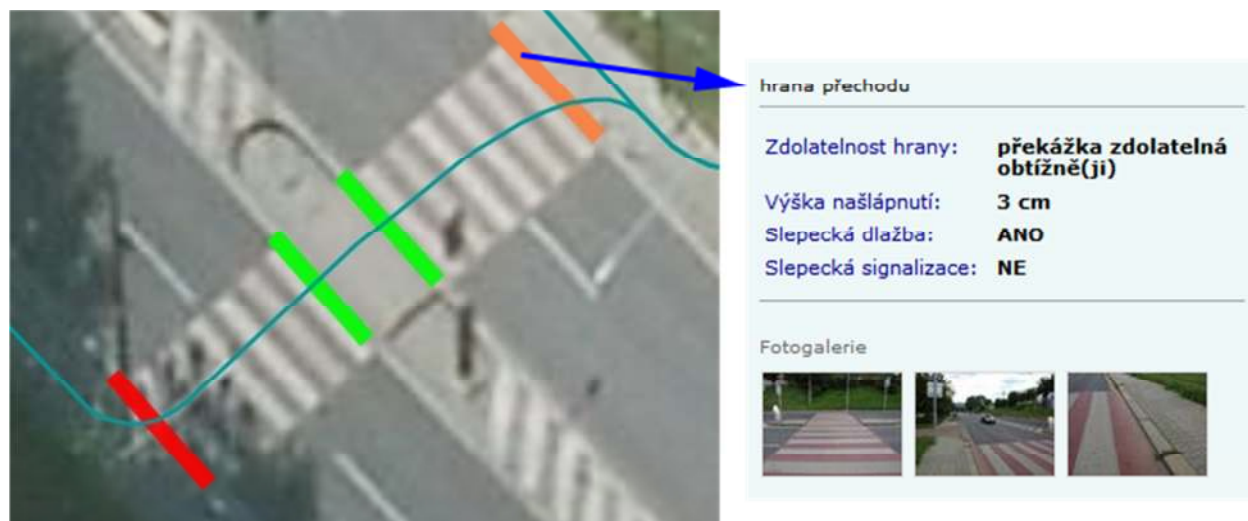
Figure 12 - Height of barriers marked on a pedestrian crossing
