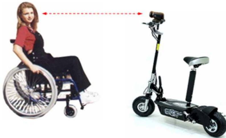
Figure 2 – Electric scooter utilised for shooting of videos from the wheelchair person's point of view.
