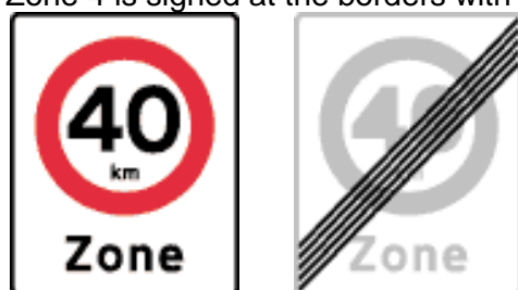
Figure 17: E68.4 sign “Zone with local speed reduction” (to the left) and E69.4 sign “End of the zone with local speed reduction” (to the right)
