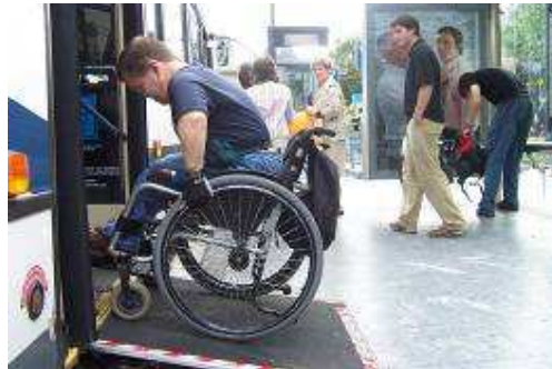
Ramp for the disabled access (wheel chairs)
