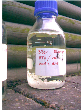
Figure 6: Deposits in B30 TME biodiesel at cold winter conditions
