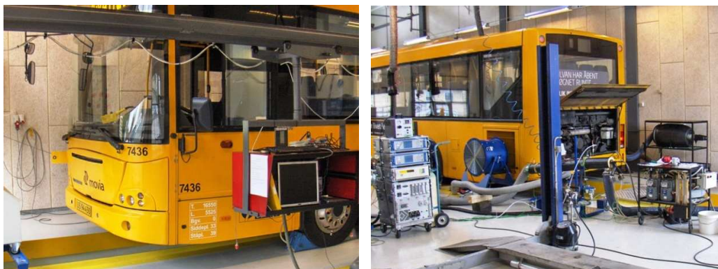
Figure 9: Example of a bus on rolling road during the 5-mode test
