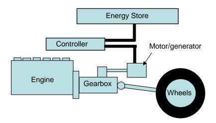
In the parallel hybrid, the system retains a physical connection between the engine and the roadwheels through a mechanical transmission with an electric motor in parallel to it. This allows the system controller to typically pull away from rest using the electric motor and subsequently blend in diesel power from the engine when the engine is operating in its 'sweet spot'.
