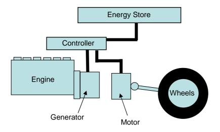
It can be seen there is no physical connection between the engine and road wheels. A good way of visualising this set up would be to consider it to be an electric vehicle with its own on board electricity generation system.
